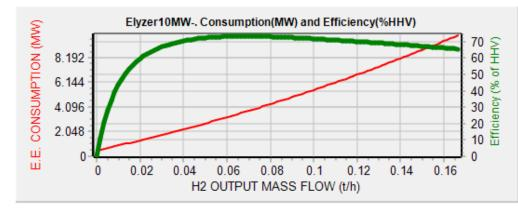
Nominal H2 mass flow = 0.166 t/h; It is needed at least 0.5 MW to generate H2
