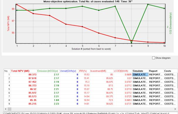
COMPONENTS: PV gen: PV10 (10 MWp)x6 (100% PV#1: slope 35%, azimuth 0%) // Batteries Bat5MWh (5 kAh): 1s. x 1p. // 3 Wind Turb. WindT1 (2 MW at 14 m/s) // Inverter Inv-Ch5MW of 5 MVA // Unmet load = 0 % // Total Net Present Value (NPV) = 88.373 M€, IRR = 15.5%.
