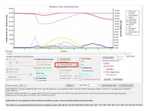
The black thin line is the energy in the H2 tank (in HHV of hydrogen). In the simulation we can see the load peak at 6 a.m., with the high H2 load to supply the car, which is taken from the H2 tank (we can see the H2 tank energy is reduced in 11.82 kWh, corresponding to 0.3 kg of H2). Later, when the electrolyzer generates H2, the H2 tank energy increases as it stores the H2 generated.
