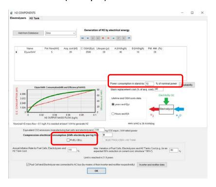
In high power projects, by default there is no Fuel cell considered in the system ("FUEL CELL" checkbox is unchecked), we have just electrolyzer. Also by default no H2 tank is considered (all the hydrogen generated will be sold).
